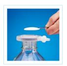
1. Place base on the receiving vessel.\* Place the membrane on the clean, dry filter support.
