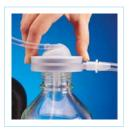
**5**. Apply vacuum to pull liquid through the filter.
