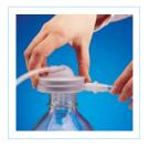
3. Attach vacuum tubing from vacuum source to the vacuum port adapter on the housing base.
