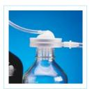
**4**. Place feedline tubing into solvent to be filtered.
