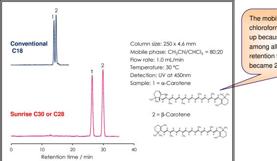
The mobile phase including chloroform makes alkyl chains brash up because chloroform can enter among alkyl chains. Consequently retention times of C30 or C28 became 2 times longer than C18.
