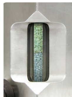
AFS Purifier I; oxygen and moisture indicator
