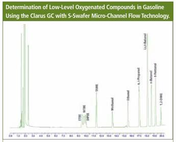
Column: Elite-1, 15 m x 0.530 mm x 1.5 µm Part No. **N9316046** S-Swafer Part No. **N6520272**
