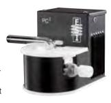
signal stability, reducing polyatomic interferences such as oxides, and reducing solvent loading when volatile organic solvents are analyzed. The PC³ has two present temperatures +2 °C / -5 °C and is ideal for analysis of aqueous or aqueous/organic mixtures. The PC³-LT operates at +2 °C / -20 °C to reduce the solvent load on the plasma for analysis of 100% volatile organic solvents.
