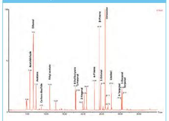
Recommended Column: Elite-5ms, 60 m x 0.25 mm x 1.0  $\mu$ m, Part No. N9316287
