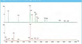
Column: Elite-5ms column, 30 m x 0.25 mm x 0.25  $\mu$ m, Part No. **N9316282** Liner Deactivated Liner, Part No. **N6502002**
