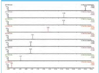
Recommended Column: Elite-35ms, 30 m x 0.25 mm x 0.25  $\mu m$  (Part No. N9316438)
