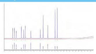
Recommended Column: Elite-1, 30 m, 0.32 mm, 3.0 μm, Part No. **N9316025**
