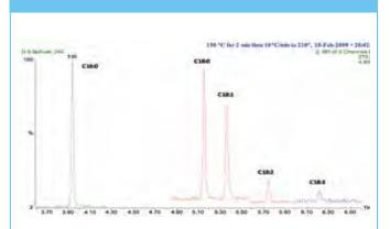
Recommended Column: Elite-23, 50 m x 0.25 mm x 0.25 μm, Part No. N9316506
