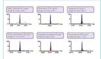
Recommended Column: Elite-624, 60 m x 0.25 mm x 1.4 μm, Part No. **N9316006**
