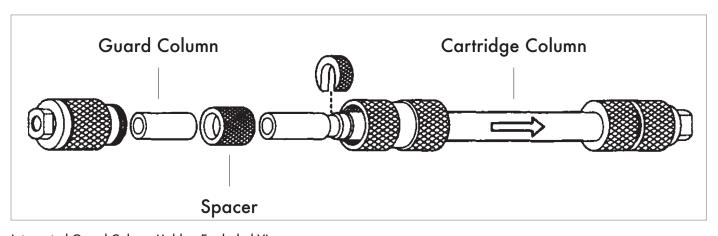
Integrated Guard Column Holder, Exploded View
